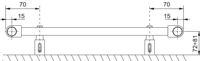
The mounting set is delivered as standard and consists of 4 special plastic brackets, screws, dowels and assembly instructions.
